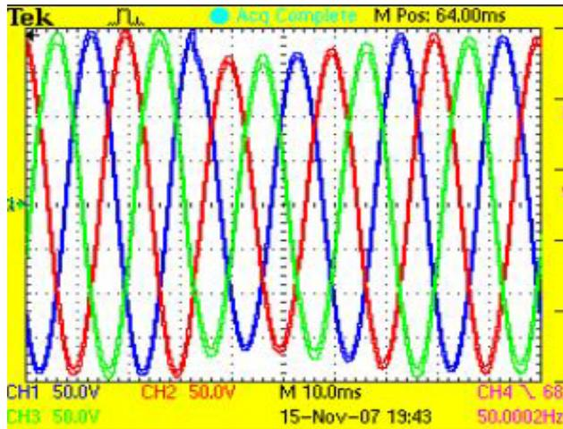
Fig. 9. Load voltage transients during voltage sag (experiment)
