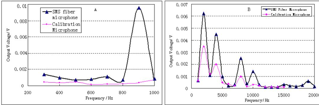
Fig.5 Frequency response comparison of SMS fiber sensor to calibration microphone at low frequency (A-below 1 KHz) and high frequency (B-1 KHz to 20 KHz)
