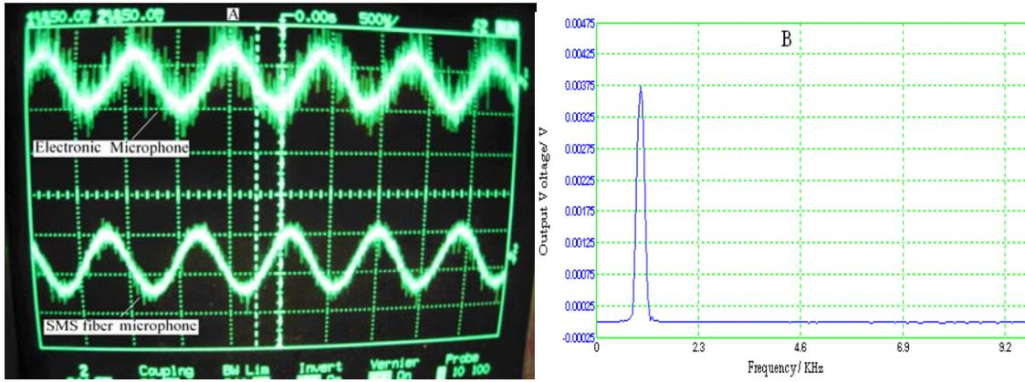
Fig.4. Detected acoustic signal of SMS fiber microphone at 1 KHz (a-time domain and b-frequency domain)
