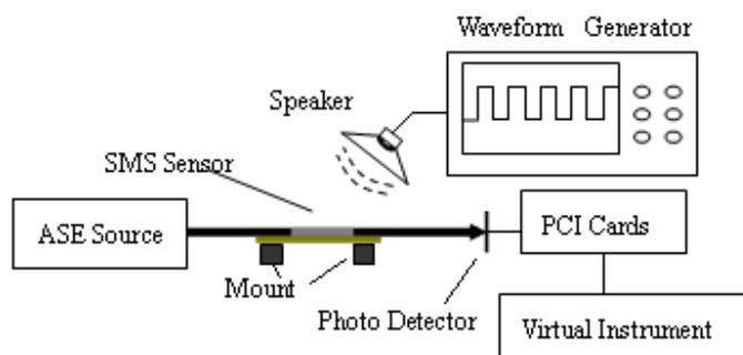
Fig.3. Experimental setup of SMS fiber microphone system
