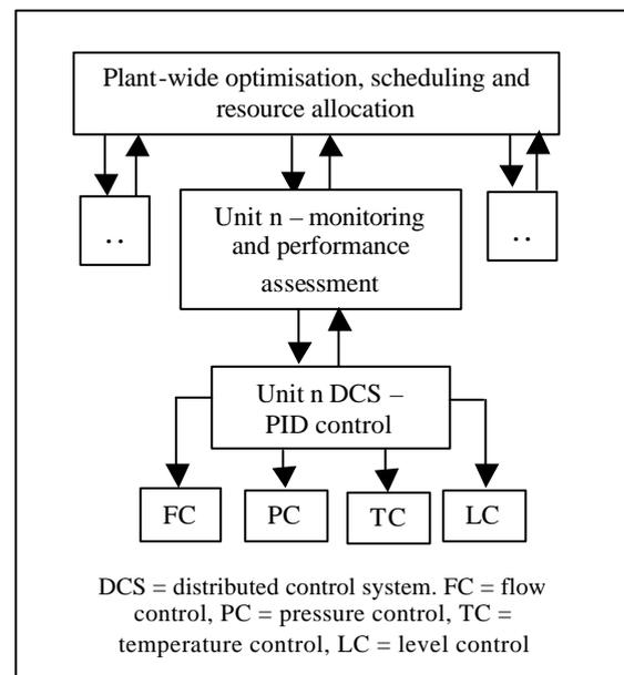
Figure 1: Hierarchical integrated enterprise wide control scheme
