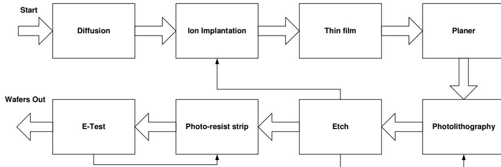
Figure 2: Basic operation sequence for wafer fabrication
