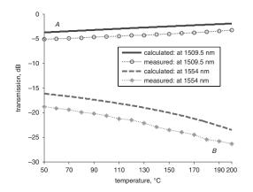
Fig. 3 Transmission of SMS structure against temperature at wavelengths of 1509.5 and 1554 nm
