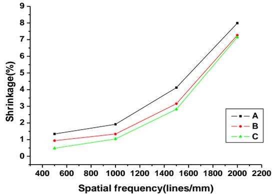
Fig. 6. Dependence of shrinkage on spatial frequency for recording intensities A (-■-) 1 mW/cm<sup>2</sup>, B (-●-) 5mW/cm<sup>2</sup>, C (-▲-) 10 mW/cm<sup>2</sup> for  $60 \pm 5 \mu\text{m}$  layers.
