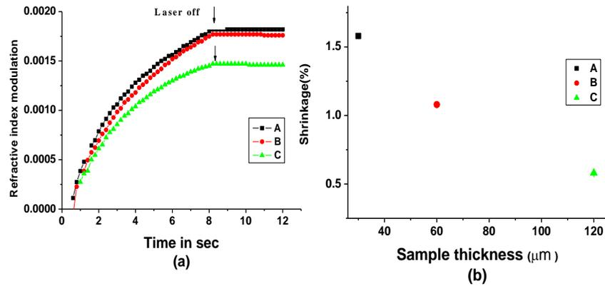
Fig. 8. Dependence of refractive index modulation with exposure time (a) and percentage shrinkage on sample thickness (b) for thickness A (■) -30 $\mu\text{m}$ , B (●) -60 $\mu\text{m}$ , C (▲)-120 $\mu\text{m}$ .
