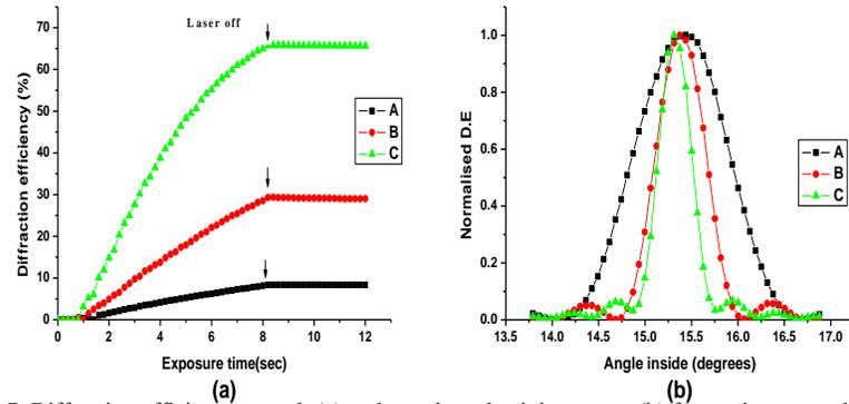
Fig. 7. Diffraction efficiency growth (a) and angular selectivity curves (b) for gratings recorded in layers of thickness A (-■-) 30  $\mu\text{m}$ ; B (-●-) 60  $\mu\text{m}$ , C (-▲-) 120  $\mu\text{m}$ . The corresponding position of Bragg peak in (b) are A (-■-) 15.441°, B (-●-) 15.375°, C (-▲-) 15.31°.
