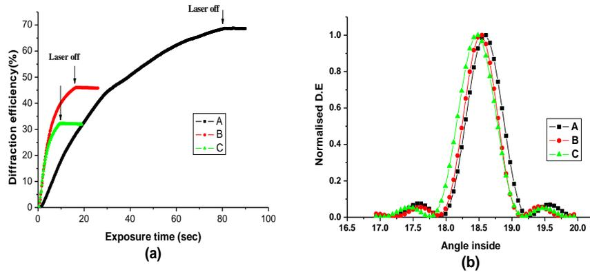
Fig. 2. Diffraction efficiency growth (a) and angular selectivity curves (b) for gratings recorded at A(-■-) 1mW/cm<sup>2</sup>, 80sec; B (-●-) 5mW/cm<sup>2</sup>, 16sec, C (-▲-) 10mW/cm<sup>2</sup>, 8sec. The corresponding peak positions in (b) are A (-■-)18.525°; B (-●-)18.483°; C (-▲-) 18.468°.
