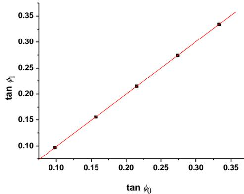
Fig. 5. Dependence of the new slant angle on the initial slant angle for recording intensity 10mW/cm<sup>2</sup> . at 1000 lines/mm, shrinkage-1.08%.
