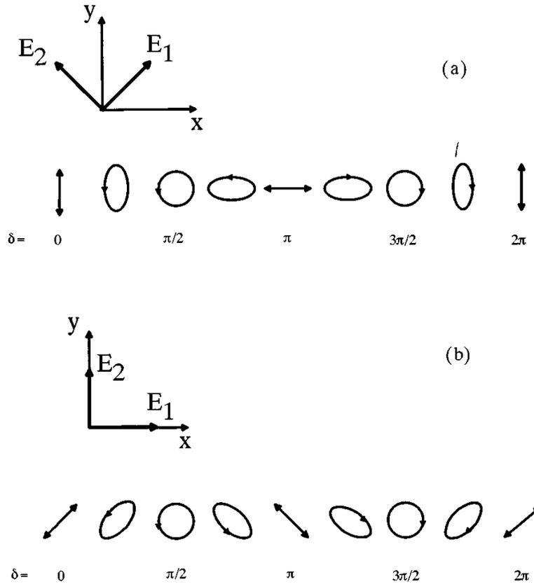
Fig. 4. Polarization modulation of the interference light field recording the gratings in the two geometries used, (a) and (b).  $E_1$  and  $E_2$  are the polarization vectors of the two recording waves, and  $\delta$  is the phase difference between them.
