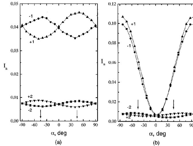
Fig. 2. Experimentally measured dependencies of the normalized intensity  $I_n$  (the diffraction efficiency) of the waves diffracted in the  $+1$ ,  $-1$ ,  $+2$ , and  $-2$  orders on the polarization azimuth  $\alpha$  of the reconstructing He-Ne beams. The arrows show the azimuths of the recording beams polarizations:  $-45^\circ$  and  $+45^\circ$ . The recording intensity is  $100 \text{ mW/cm}^2$  [Fig. 2(a)] and  $750 \text{ mW/cm}^2$  [Fig. 2(b)].
