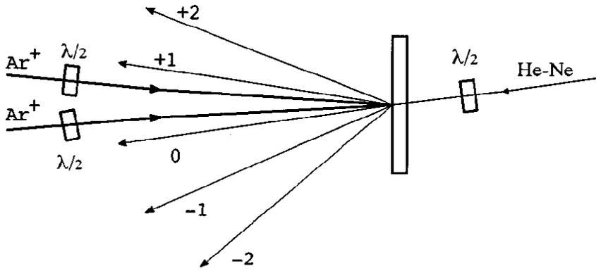
Fig. 1. Geometry of the recording and diffracted beams.
