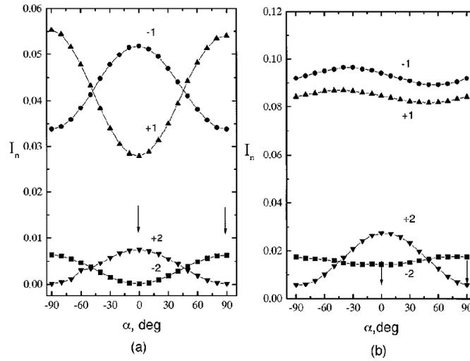
Fig. 3. Experimentally measured curves  $I_{\pm 1}(\alpha)$  and  $I_{\pm 2}(\alpha)$  in the case in which the recording waves are with horizontal ( $0^\circ$ ) and vertical ( $90^\circ$ ) polarizations. The recording intensity is  $150 \text{ mW/cm}^2$  [Fig. 3(a)] and  $600 \text{ mW/cm}^2$  [Fig. 3(b)].
