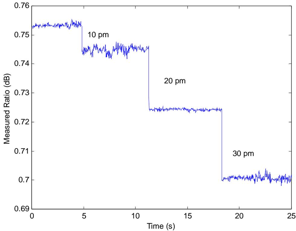
**Figure 5** Measured ratio as the wavelength is tuned
