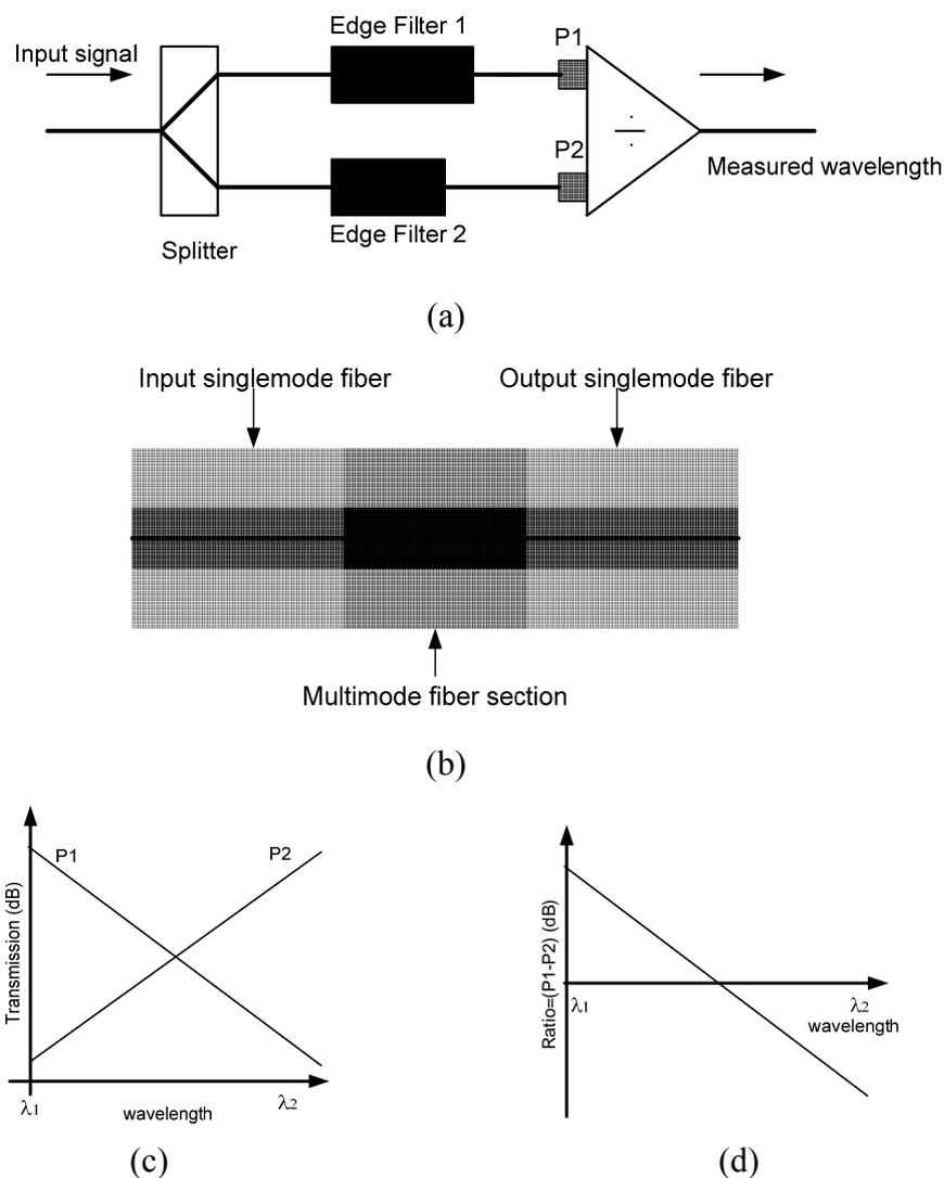
**Figure 1** Schematic structure of (a) a ratiometric wavelength measurement system (b) an SMS fiber-based edge filter (c) the desired spectral response of the two edge filter arms and (d) the output ratio between the two arms.
