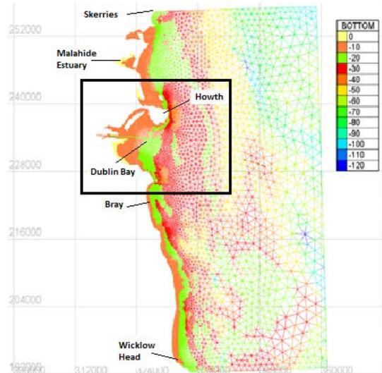
Fig 3. Mesh and Bathymetry of East Coast Model
