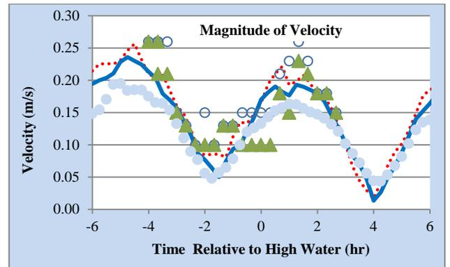
Fig 15. Amplitudes of Tidal Currents at Station 8
