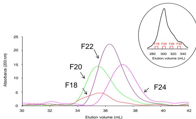
**Fig. 4.** SEC-HPLC chromatogram of fractions of sCT-P<sub>6.5kDa</sub> purified by IE-FPLC. The corresponding IE-FPLC chromatogram is also shown for reference (inset).
