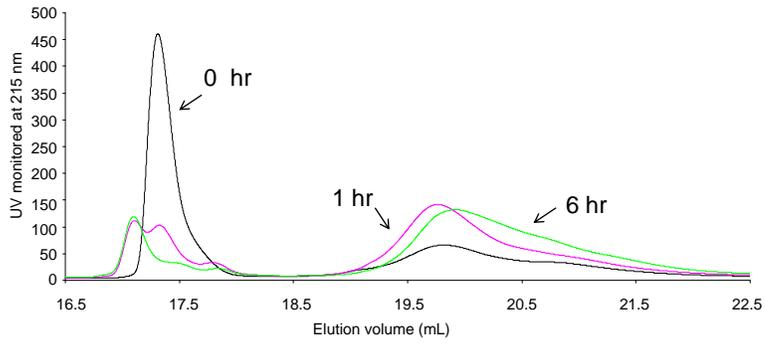
**Fig. 2.** RP-HPLC spectra following the conjugation reaction of sCT with P to yield a 9.5kDa conjugate.
