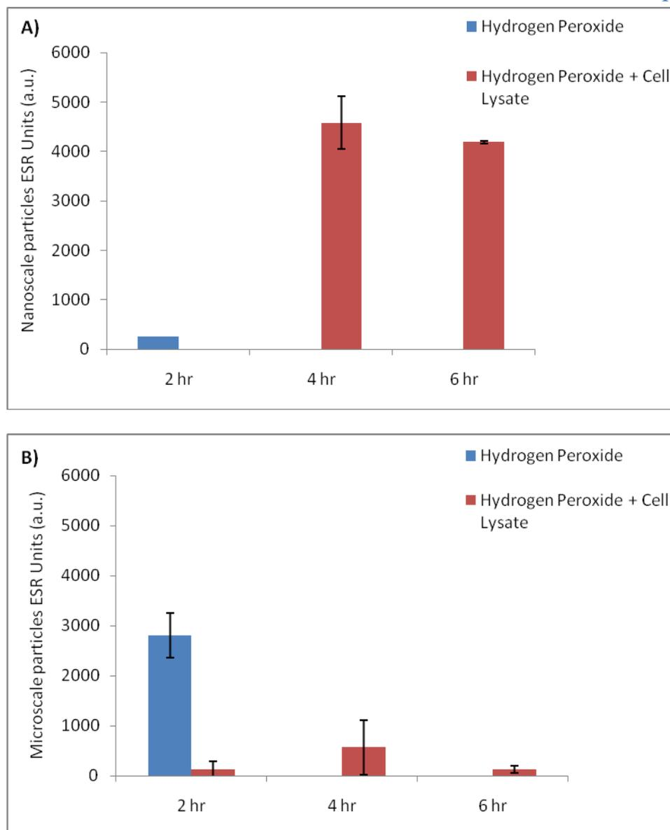
**Figure 3:** Acellular hydroxyl radical measurement on the surface of  $\alpha$ -Fe<sub>2</sub>O<sub>3</sub> nano- (A) and microscale particles (B) using spin trap, 5, 5-dimethyl-1-pyrroline-N-oxide with electron spin resonance (ESR) spectrometry. The particles were suspended in MilliQ water and cell lysate proteins (450  $\mu$ g/ml) along with hydrogen peroxide (120 mM) treatment. The measurements were taken at time points of 2, 4 and 6 h post-suspension.
