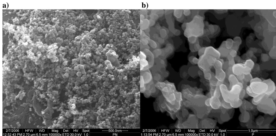
**Figure 1:** Scanning electron microscopy images of Fe<sub>2</sub>O<sub>3</sub> (a) nano- and (b) microscale particles.
