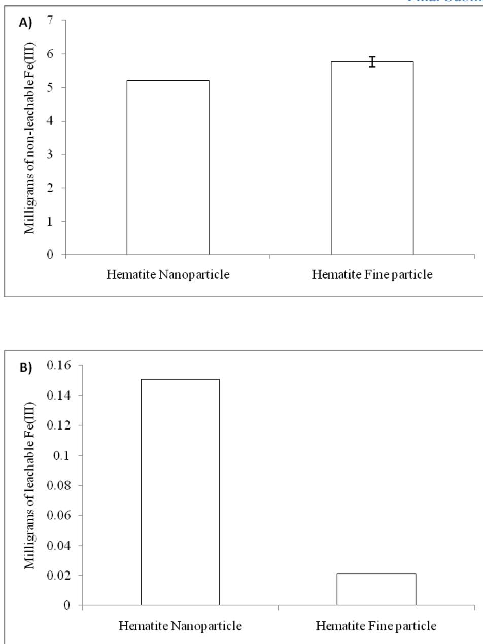
**Figure 2:** 1,10-Phenanthroline-chloride spectroscopy-based determination of non-leachable (A) and leachable Fe(III) (B) in Fe<sub>2</sub>O<sub>3</sub> nano- and microscale particles. Fe(III) concentrations determined using standard curve of Fe<sub>2</sub>Cl<sub>3</sub>.
