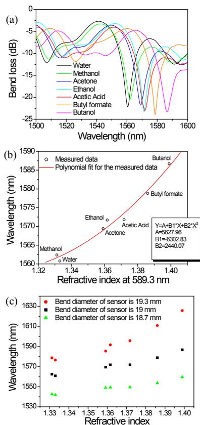
Fig. 5. (a) Transmission spectra of the fiber sensing device in a range of organic solvents; (b) 1<sup>st</sup> resonance peak shifts as a function of corresponding RI (at 589.3nm); (c) the peak wavelength shifts versus RI.
