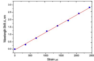
Fig. 5. Measured FBG wavelength shift with applied strain.
