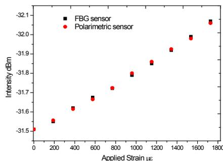
Fig.7. Strain response of both polarimetric and FBG sensor in the hybrid configuration.
