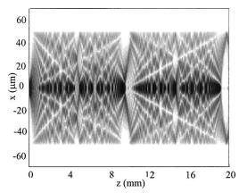
Fig. 2. Amplitude distribution of the propagation field within the multimode fiber section.
