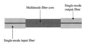
Fig. 1. Configuration of the proposed refractometer.
