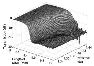
Fig. 3. Transmission losses versus length of MMF and refractive index.
