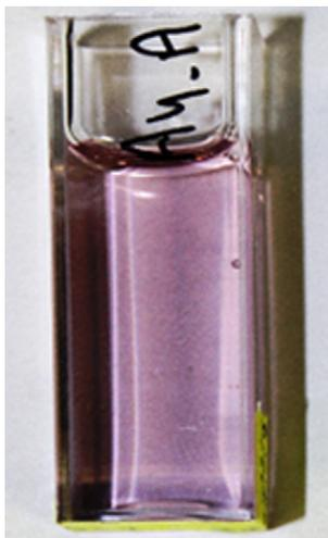
**Fig. 2.** Au NPs (50.0 ppm) dispersed in epoxy and cast in a 1 cm path length PMMA cuvette.
