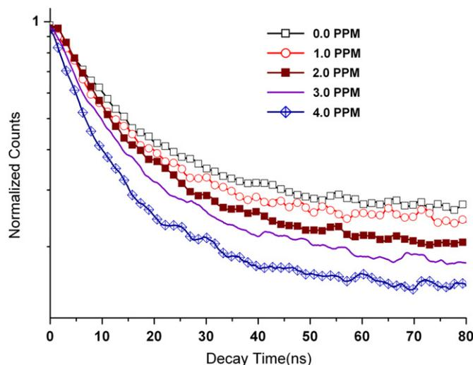
**Fig. 8.** Normalized fluorescence lifetime decay profile for the QD 570 quantum dots with varying Au NP concentrations (0.0–4.0 ppm) in epoxy. (Note: the 1.5, 2.5, and 3.5 ppm data have not been shown in this figure to keep clarity in figure).
