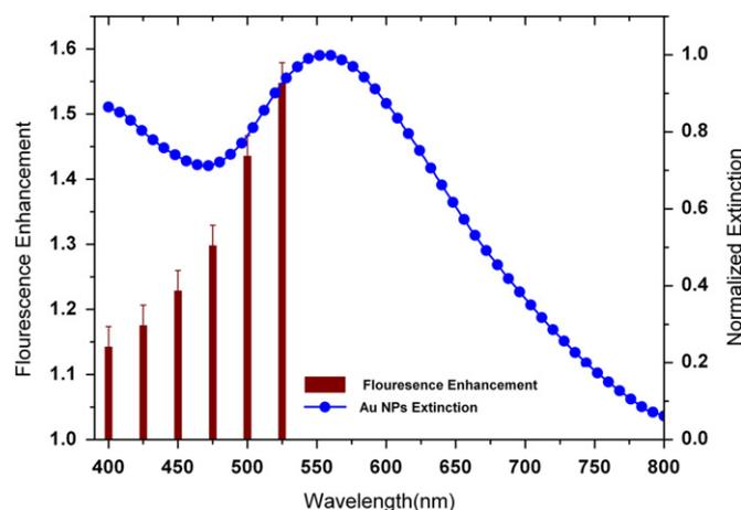
**Fig. 9.** Fluorescence enhancement as a function of excitation wavelength for the 2.0 ppm sample. Excitation enhancement was obtained by taking the ratio of the total emission of the 2.0 ppm sample to that of the 0.0 ppm sample at the particular excitation wavelength (solid bar). The normalized extinction spectra (solid circles) of the Au NPs are also plotted to illustrate the origin of the effect.
