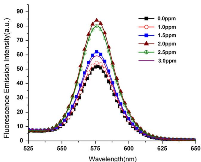
**Fig. 6.** Fluorescence emission spectra of the QD 570 quantum dots with varying Au NP concentration (0.0–4.0 ppm) in epoxy. The samples were excited at 500 nm and the emission collected at a 90° angle to the excitation beam. (Note; the 3.5 and 4.0 ppm data have not been shown in this figure to keep clarity. All data are shown in Fig. 7).
