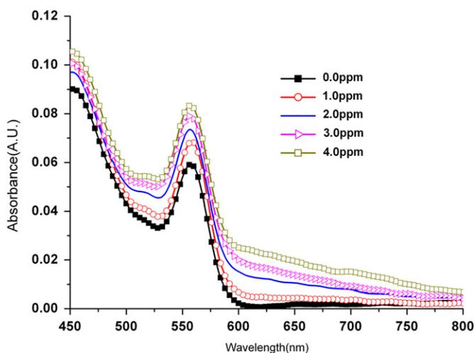
**Fig. 5.** UV-vis absorption spectra of the QD 570 quantum dots with varying Au NP concentration (0.0–4.0 ppm) in epoxy. (Note; the 1.5, 2.5, and 3.5 ppm data have not been shown in this figure to keep clarity.)
