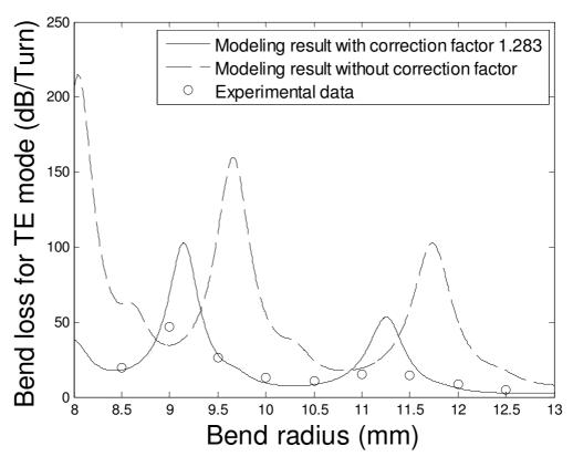
Fig. 2 Calculated and measured macrobending loss for different bending radii at 1550 nm
