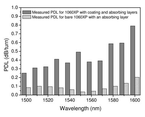
Fig. 7 Measured PDLs for bend radius of 10.5 mm (one turn)
