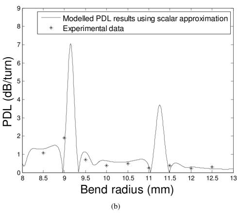
Fig. 5 (a) Calculated bend loss for TE and TM mode for different bend radii (correction factor is 1.283 at 1550 nm wavelength); (b) theoretical and experimental differences in bend loss between TE and TM mode for 1060XP fiber with different bend radii
