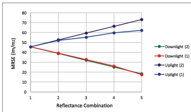
**Figure 3. Plot of MRSE levels based on Duff's comparison<sup>11</sup> of downlight and uplight luminaires calculated by exact formula (1) and approximate formula (2). The room characteristics are as described previously, and in every case the luminaire emits the same level of luminous flux.**
