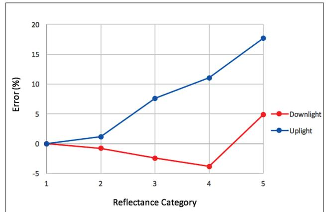
**Figure 2. Levels of error incurred using formula (2) rather than formula (1) in Duff's comparison<sup>11</sup> for downlight and uplight luminaires illuminating a room with the five reflectance combinations shown in Table 1.**
