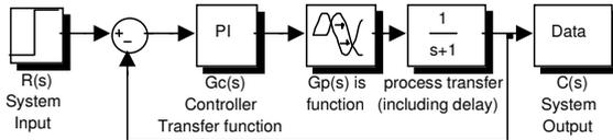
Figure 1: Block diagram of standard feedback control system.
