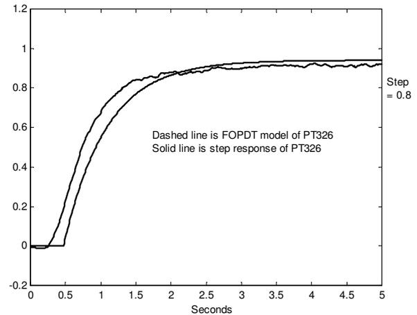
Figure 9. Open loop step response of Process Trainer PT326 and FOPDT model of PT326.
