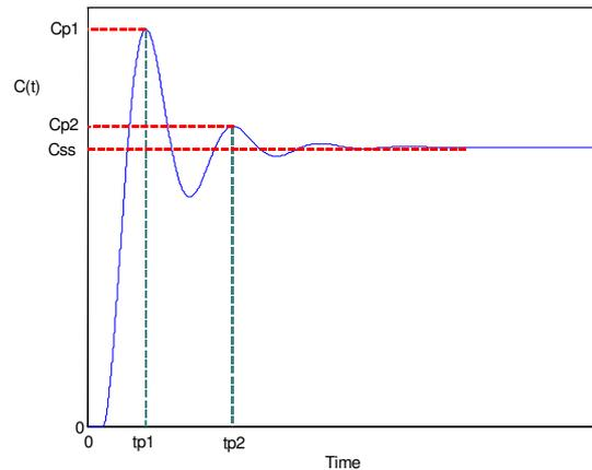
Figure 2: Typical under-damped closed-loop step response under PI control.
