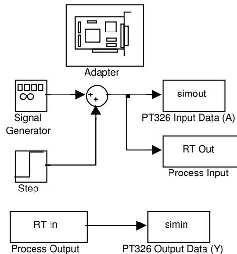
Figure 10. File used to determine frequency response of Process Trainer PT326.
