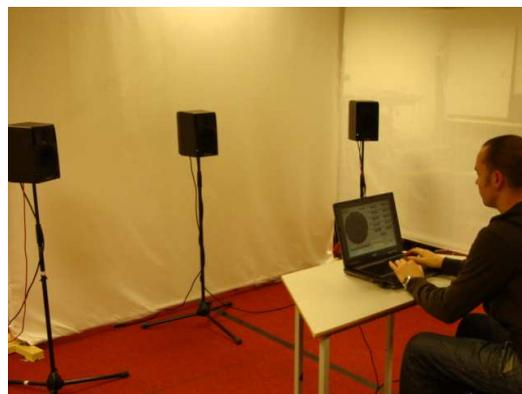
Figure 6: Listening Test Configuration. Bottom: Participant in the listening environment conducting the perceptual experiment with dedicated test software.
