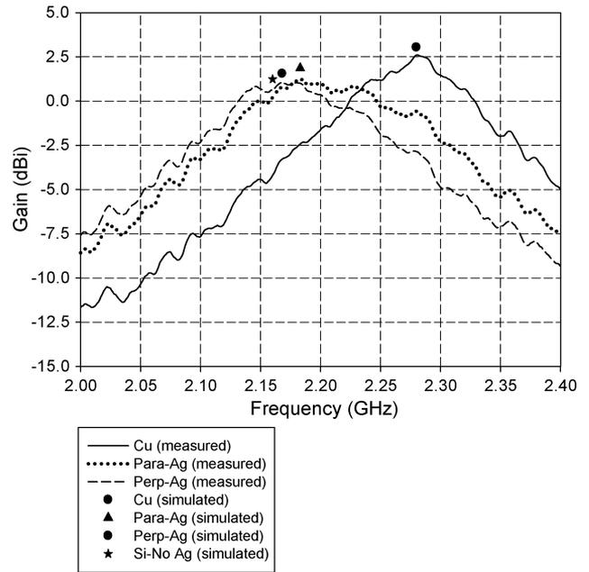
Fig. 4. Simulated and measured gain for the solar antenna configurations.
