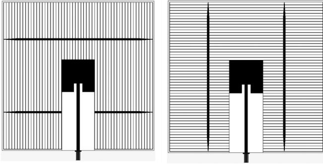
Fig. 2. Electrode lines alignment with the microstrip feed line: parallel (left) and perpendicular (right).
