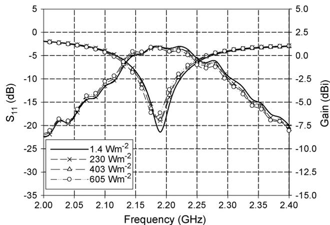
Fig. 6. Variations of parallel solar antenna  $S_{11}$  and Gain with different light intensity values.
