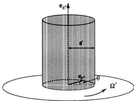
FIG. 1. Geometry of the single semi-infinite circular cylinder of radius  $a'$  with a rotating end wall, of angular velocity  $\Omega'$  about the axis of symmetry, relative to a cylindrical polar coordinate system  $(r', \theta, z')$ .
