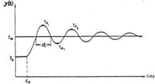
Figure 3. Under-damped transient response, for a step input [3].
