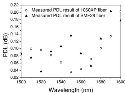
Fig. 6 Measured PDL in wavelength ranging from 1500nm to 1600 nm for bare 1060XP fiber coated with an absorbing layer (circles) and SMF28 fiber with coating and absorbing layers (solid triangle).
