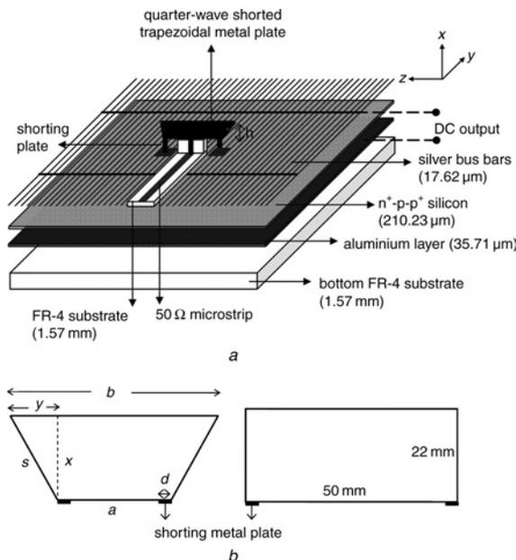
**Fig. 1** Expanded layout of proposed quarter-wave trapezoidal metal plate solar antenna, and topology of quarter-wave trapezoidal RF radiating element and its equivalent quarter-wave rectangular metal plate
