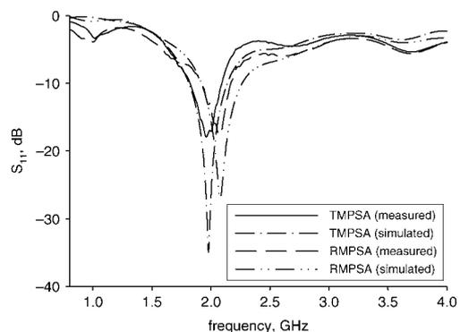
**Fig. 2** Measured and simulated  $S_{11}$  of solar antennas
