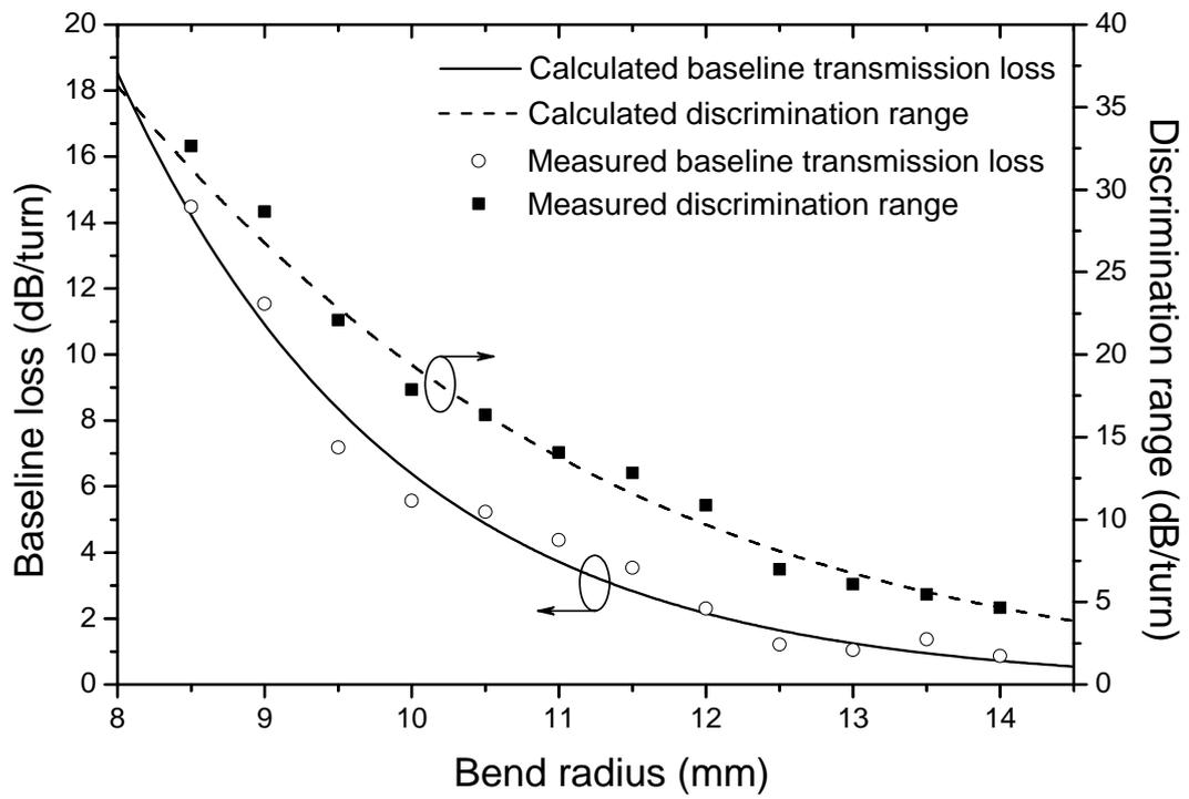
Fig.2. Calculated and measured baseline transmission loss and discrimination range as a function of bend radius for 1060XP fiber with an absorbing layer, the fiber length is 1 turn.
