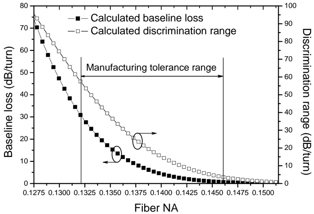
Fig.4. Calculated baseline transmission loss and discrimination range as a function of fiber core NA for 1060XP fiber with an absorbing layer, the fiber bend radius is 10.5 mm, and length is 1 turn.
