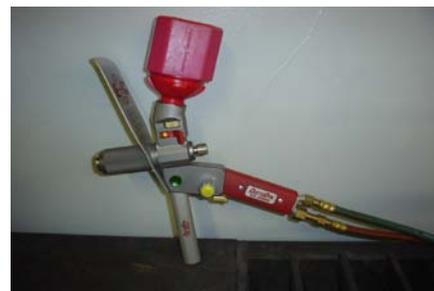
Figure 2 CDS 8000 Flame Spray gun
