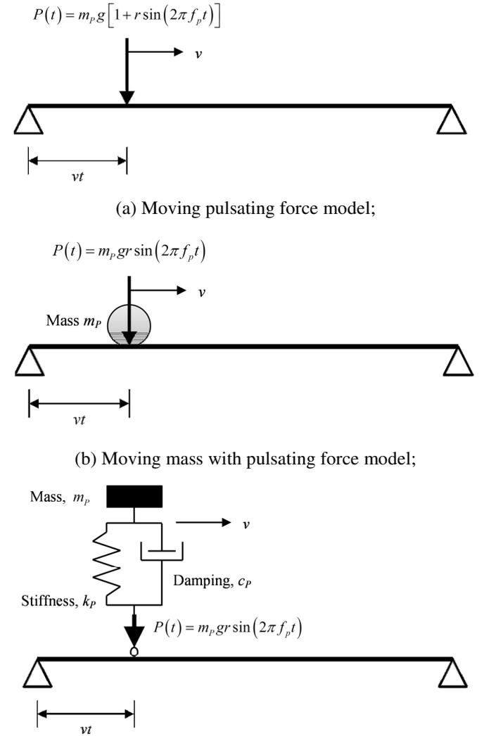
(c) Moving spring-mass-damper with pulsating force model;
