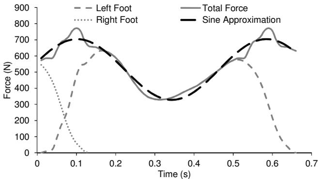
Figure 6. Typical vertical ground reaction force and approximated model force.
