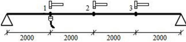
Figure 2. Location of accelerometers and impacts.
