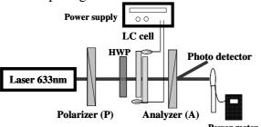
**Fig. 1** Optical setup used to characterize the twisted nematic LC device
