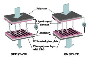
Fig 2 Operation of the twisted nematic LC device
