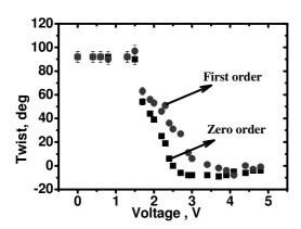
Fig 5 Twist angle verses voltage
