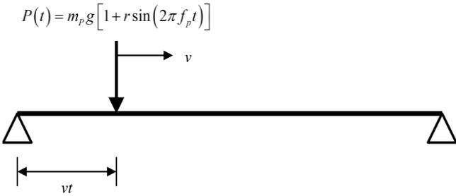
Figure 2. Moving pulsating force model of a pedestrian.
