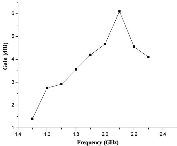
Figure 5 The variation of maximum gain for the proposed antenna
