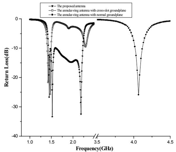
Figure 2 Comparison of three different annular-ring patch antennas
