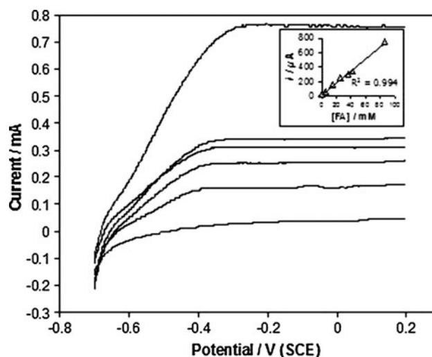
**Fig. 2** Linear sweep voltammery at a  $\text{TiO}_2$ -coated CI electrode (area =  $25$  cm $^2$ , swept at  $50$  mV/s) of aqueous  $0.1$  M KCl with incremental amounts of FA added with exposure to a  $150$  W Xe lamp. Photocurrent increases with FA concentrations of  $0$ ,  $15$ ,  $25$ ,  $36$ ,  $42$ , and  $85$  mM
