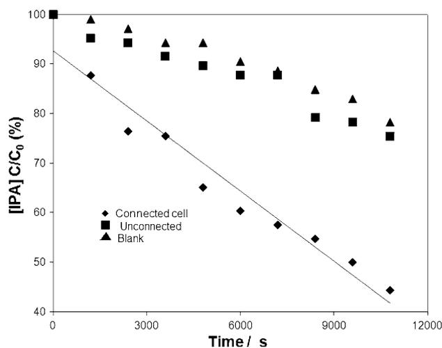
**Fig. 4** Photodegradation of IPA (13.9 mM) in aqueous 0.1 M KCl over 3 h in a one compartment cell. The advantages of the PEC cell compared to the unconnected TiO<sub>2</sub>/CI electrode are evident. 25 cm<sup>2</sup> TiO<sub>2</sub>/CI anode and air cathode connected through a 1 kΩ resistor. Unconnected cell and blank are also included. Irradiated by a 150 W Xe lamp
