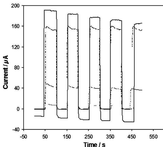
**Fig. 3** In situ transient photocurrent-time profile in order of increasing concentrations (— = 0 mM, --- = 1 mM, - - = 10 mM, — = 100 mM) of aqueous FA in 0.1 M KCl on intermittent exposures to a 60 W tungsten lamp. 25 cm<sup>2</sup> TiO<sub>2</sub>/CI anode and 1.3 cm<sup>2</sup> air cathode were used. Current was collected for 500 s with a Pico technology ADC-16 data logger across a 1 kΩ resistor
