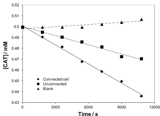
**Fig. 6** Degradation of CAT (0.5 mM) in aqueous 0.1 M KCl.  $\text{TiO}_2$ -coated CI electrode is the anode ( $25 \text{ cm}^2$ ) while an air cathode was used. Irradiated by daylight for 3 h. It is shown that the PEC cell can work competently with low irradiance
