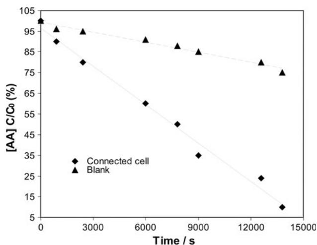
**Fig. 7** Degradation of AA (60 μM) in aqueous 0.1 M KCl. 60 W tungsten household lightbulb was the light source. PEC cell as in Fig. 3. For the PEC cell there is almost complete photodegradation of organic within 4 h
