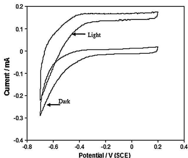
**Fig. 1** Cyclic voltammery of FA (16 mM in aqueous 0.1 M KCl) in dark and light (150 W Xe lamp) conditions cycled positively from  $-0.7$  to  $0.2$  V (SCE) at  $50$  mV/s. The working electrode is a  $\text{TiO}_2$ -coated CI electrode ( $25$  cm $^2$ )
