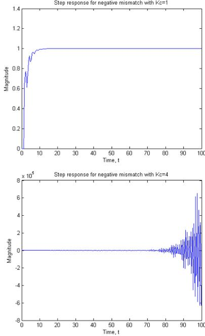
is not practically realisable, since along with an infinite spiral, the time-delay generates loops whose number is infinite [4, 6-7].
