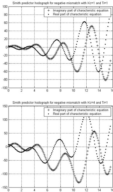
From these figures, it can be noticed that the roots interlace when  $K_c = 1$  and they do not interlace when  $K_c = 4$ . This corresponds to step response results, i.e., the closed-loop system is stable for  $K_c = 1$  and unstable for  $K_c = 4$ . It has also been noticed that the roots interlace for  $\tau_m = \tau_p$ , which again corresponds to the step response results found.
