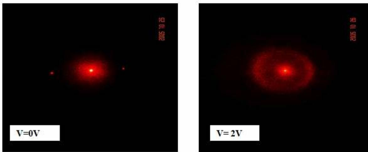
**Figure 9:** Switchable liquid crystal diffraction grating with rings
