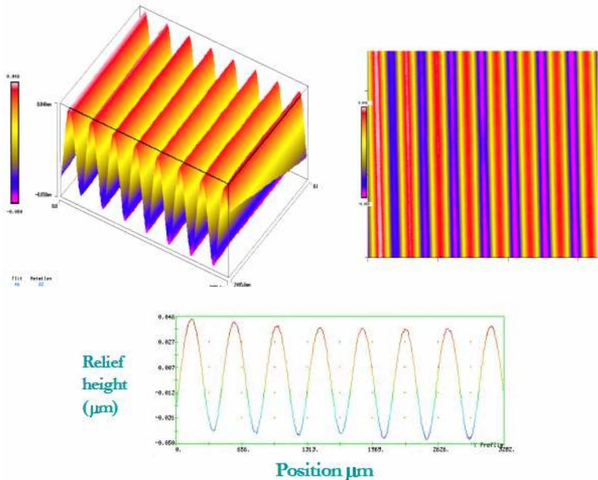
**Figure 5** Photoinduced surface relief grating inscribed in photopolymer layer at spatial frequency 100lines/mm. Recording intensity is 10mW/cm<sup>2</sup> and the recording time is 35sec.
