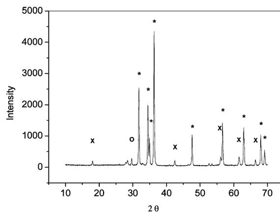
**Fig. 7** XRD of the sintered varistor prepared from nano-array ZnO sintered at 1050 °C (\* = ZnO; X = Zn<sub>7</sub>Sb<sub>2</sub>O<sub>12</sub>; O = Bi<sub>2</sub>O<sub>3</sub>).
