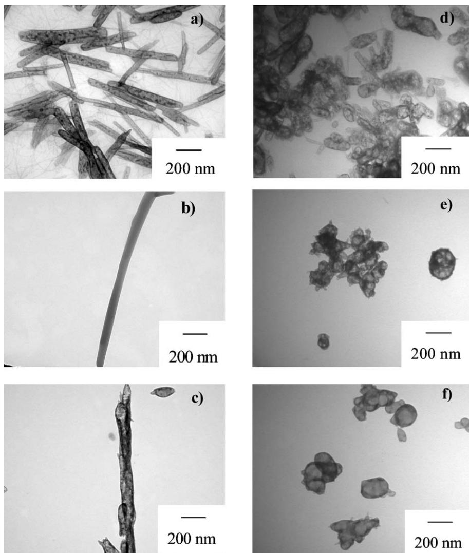
**Fig. 3** Effect of modifiers on the morphology of the products formed at various temperatures by the reaction of zinc acetate and oxalic acid. (a) Fresh gel, (b) dried at 80 °C and (c) calcined at 250 °C in the presence of modifiers (Zn : Ox : EG : DEA 1 : 2 : 2 : 0.1). (d) Fresh gel, (e) dried at 80 °C and (f) calcined at 250 °C in the absence of modifiers (Zn : Ox : EG : DEA 1 : 2 : 0 : 0).
