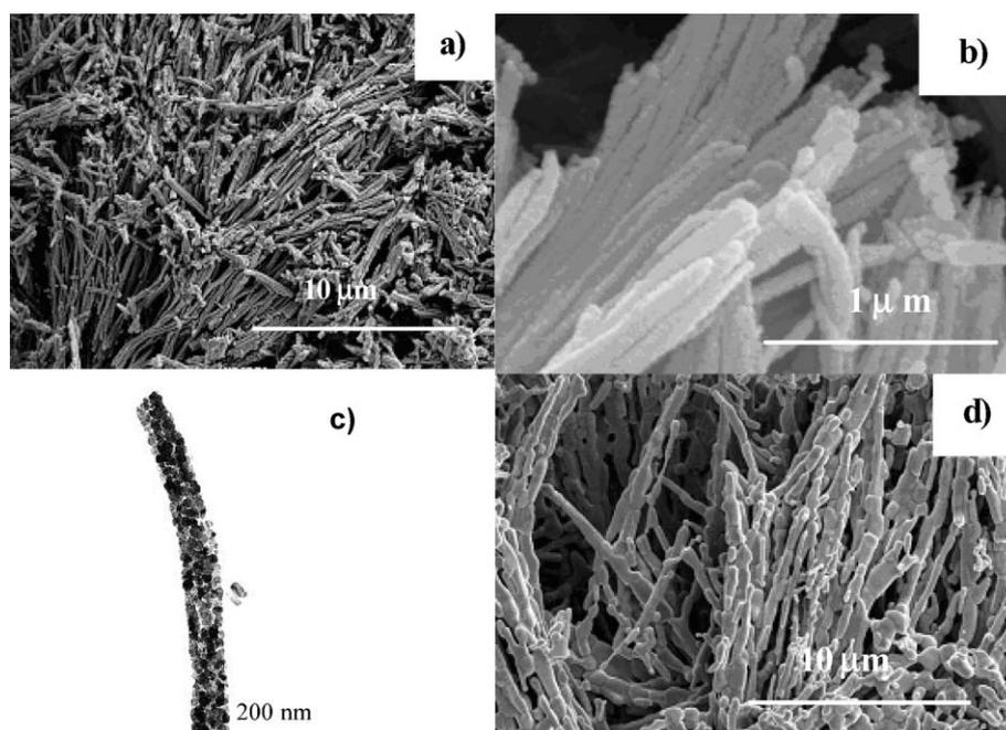
**Fig. 2** Electron microscopy images of nano-array ZnO. (a) and (b) FESEM after calcination at 500 °C; (c) TEM of a single array of ZnO nanoparticle separated by ultrasonication in ethanol; (d) FESEM of nano-array ZnO calcined at 1000 °C.
