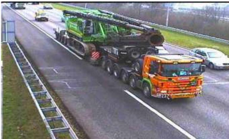
Figure 2. Vehicle with GVW of 145 t
