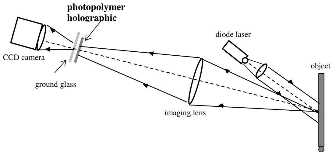
Fig.1. An optical set-up of the ESPSI system with a photopolymer grating
