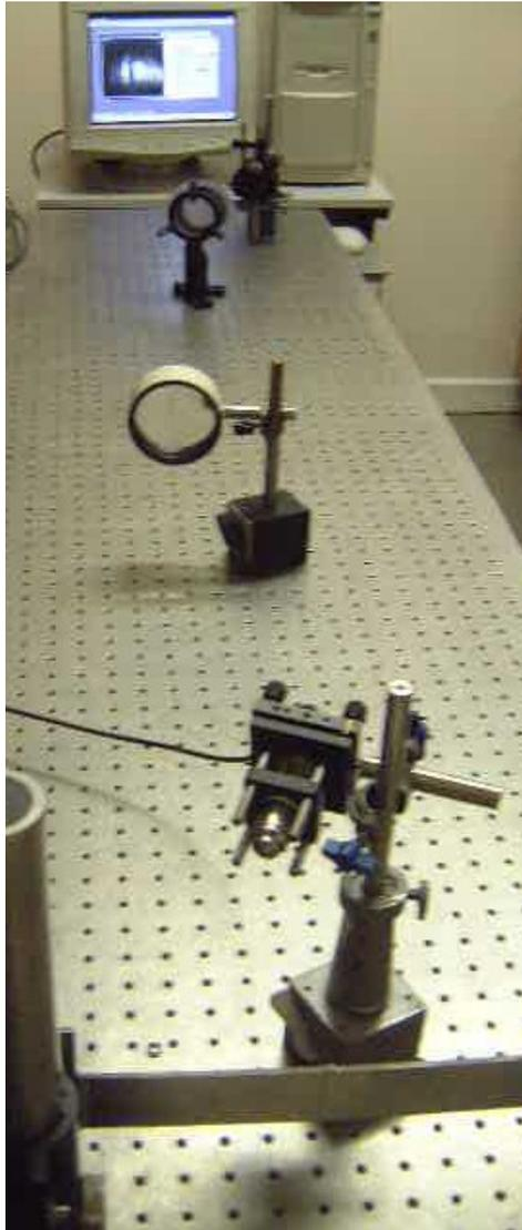
Fig. 2. Experimental set-up of the ESPSI system with a photopolymer grating
