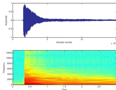
Figure 1: Spectrogram of a Piano playing C<sub>4</sub>
