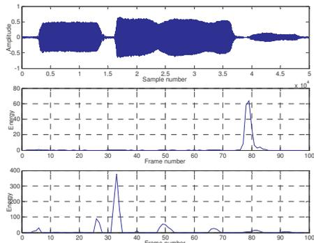
Figure 4: Excerpt of a tin whistle tune (top), D<sub>4</sub> frequency band (middle) and A<sub>4</sub> frequency band (bottom)
