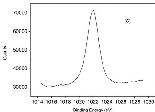
**Figure 3.** X-ray photoelectron spectra of the (a) S 2p (b) Zn2p<sub>1/2</sub> (c) Zn2p<sub>3/2</sub> peaks of ZnS450W.
