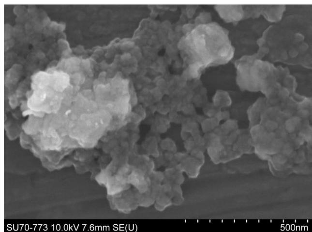
**Figure 1.** SEM image of ZnS prepared at 450 W.
