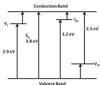
**Figure 6.** Schematic energy level diagram of ZnS
