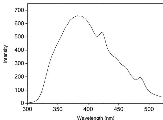
**Figure 5.** Luminescence spectra of ZnS450W excited at 275 nm.
