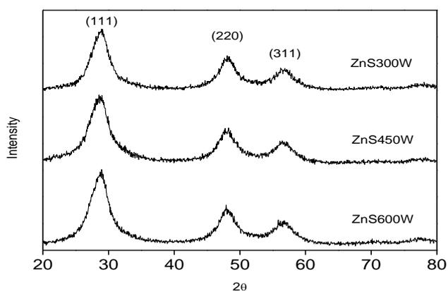
**Figure 2.** X-ray diffraction spectra of ZnS samples prepared via microwave irradiation.
