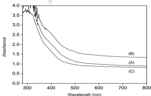
**Figure 4.** Diffuse Absorbance spectra of (A) ZnS300W (B) ZnS450W and (C) ZnS600W.
