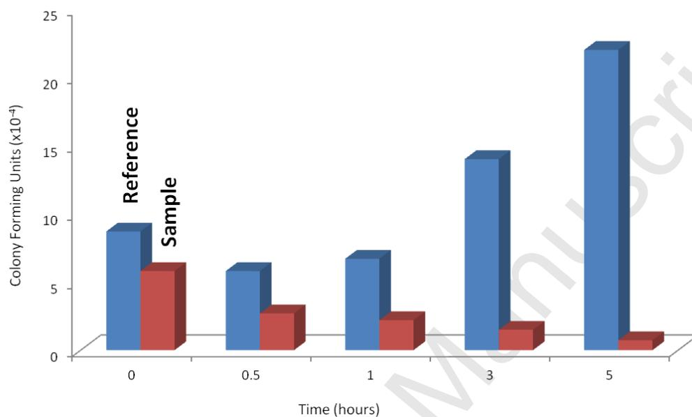
Degradation rate of the bacteria in the presence of the photocatalyst.
