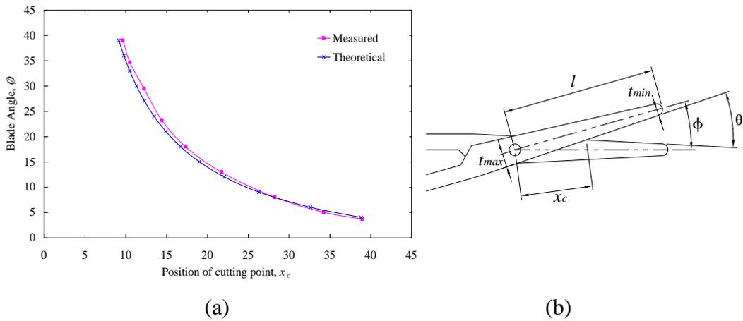
Figure 4: (a) Variation in cutting point location with angular displacement
