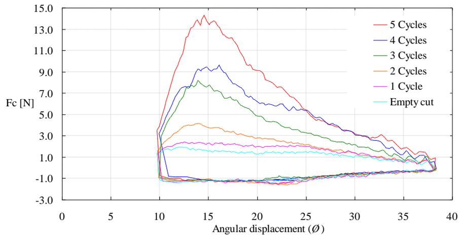
Figure 8: Force-displacement curves for five PVA samples
