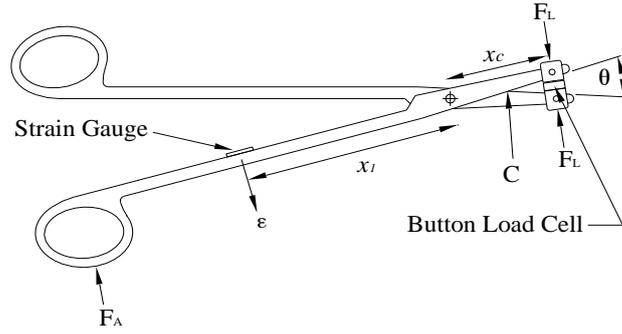
Figure 3: Scissor calibration arrangement
