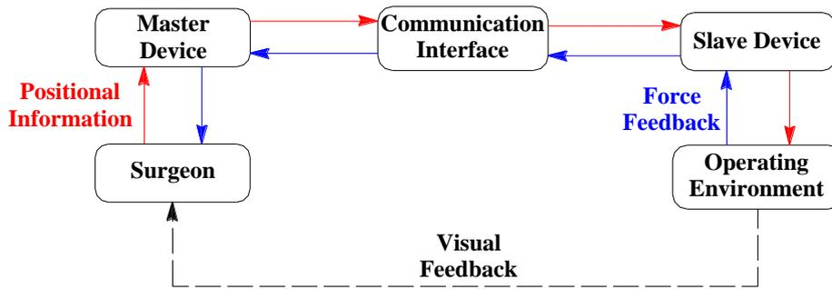
Figure 1: Typical master-slave system incorporating force feedback
