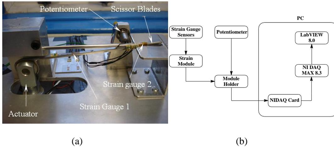
Figure 2: (a) Experimental setup (b) Data acquisition architecture
