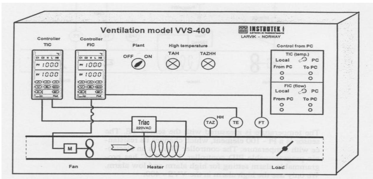
Figure 2: Three-dimensional diagram of the Instrutek VVS-400 heating and ventilation rig
