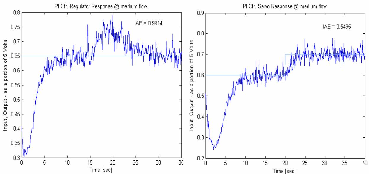
Figure 10: Responses – temperature system (with decoupling)
