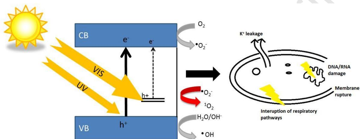
Schematic diagram of bacterial decontamination using visible light active catalyst
