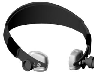
**Figure 1** Final design of hands free electrolarynx device.
