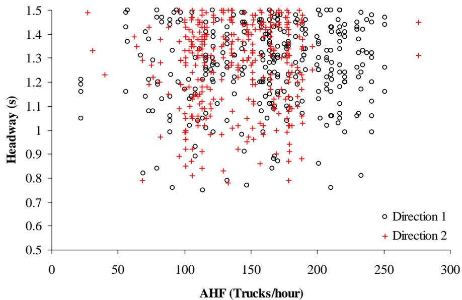
**Fig. 2 Occurrences of headways less than 1.5 seconds and corresponding average hourly flow (AHF)**
