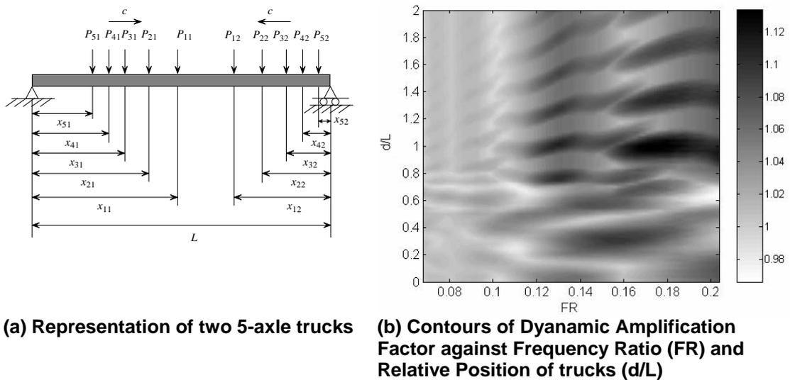
**Fig. 6 Dynamic amplification factor for two 5P-load trucks on 25 m bridge with 5% damping**
