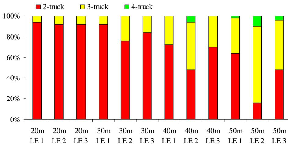
**Fig. 3 Number of trucks involved in maximum-per-day load effects (LE i = Load Effect i; LE1 & LE2 are Mid-span Moment and End Shear respectively in simply supported bridge; LE3 is Central Supported Moment in 2-span Continuous Bridge)**
