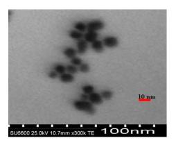
Fig.4: STEM image of Au spherical nanoparticles synthesised through reduction of HAuCl<sub>4</sub> in a PVP/EtOH mixture, in the presence of NaOH.
