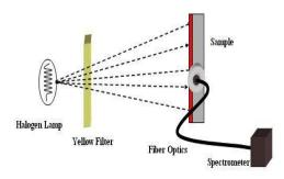
Fig.2: Experimental set for edge emission measurement.
