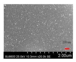
Fig.5: SEM images of spin coated Au NPs film at 1500 rpm for 30 sec.
