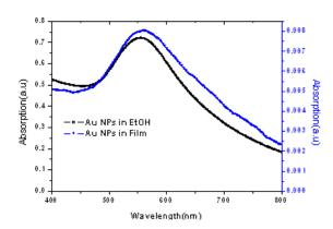
Fig.3: Absorption spectra of spherical 10±1nm Au nanoparticles in solution and in spin coated film.
