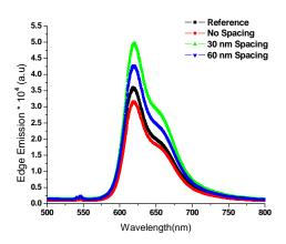
Fig.7: Edge emission for four types of samples In the case of zero spacing samples the edge emission was decreased even though a large number of dyes molecules located in the range of enhanced field. This is due to quenching of emission; mechanism may include chemical bonding and nonradiative energy transfer from
