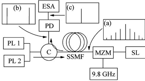
Fig. 1. Experimental setup for the generation of millimeter waves. (SL: signal laser, MZM: Mach-Zehnder modulator, PL: pump laser, PD: photodiode, ESA: electrical spectrum analyzer, C: circulator, SSMF: standard single-mode fiber.)
