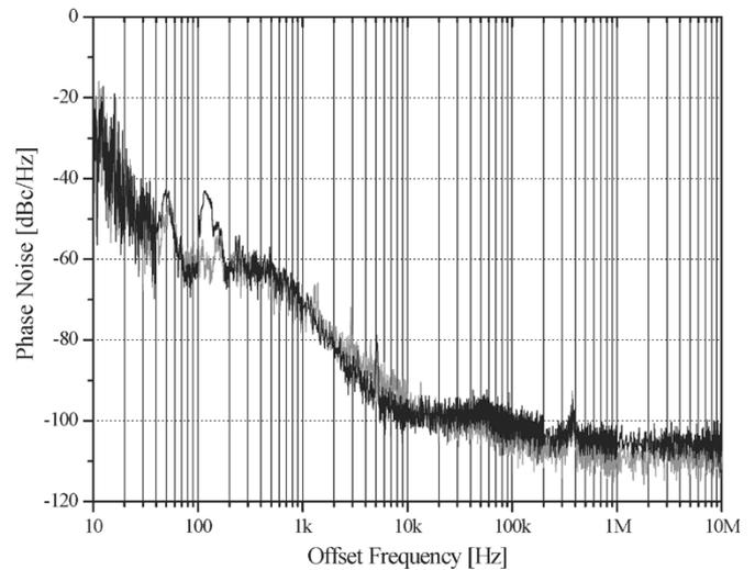
Fig. 5. Phase-noise measurement of the 39.199989-GHz signal generated by an EDFA (dark curve). At 10-kHz offset from the carrier the phase noise is  $-95$  dBc/Hz. The bright curve is phase-noise measurement of the 39.199989-GHz signal generated by SBS (see Fig. 3).
