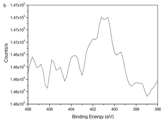
Fig. 6. N1s XPS spectra of (1:0.5) N-TiO<sub>2</sub> calcined at (a) 500 °C, (b) 600 °C.
