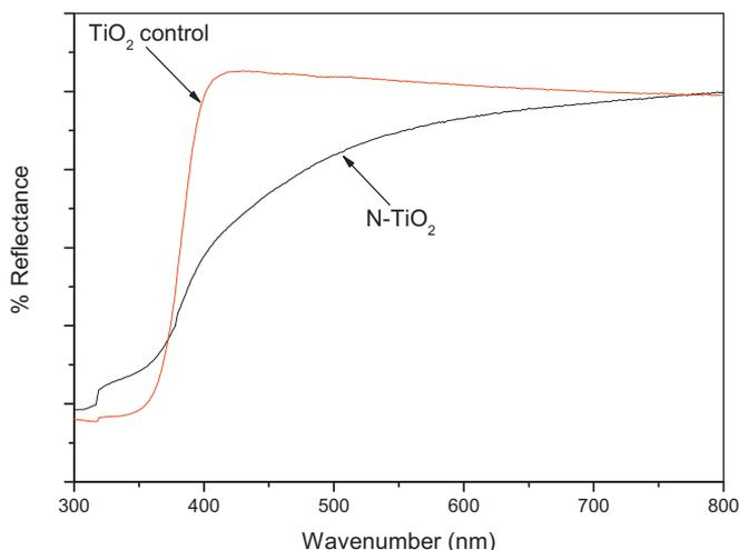
Fig. 5. Diffuse reflectance spectra of TiO<sub>2</sub> and N-TiO<sub>2</sub> calcined at 500 °C.
