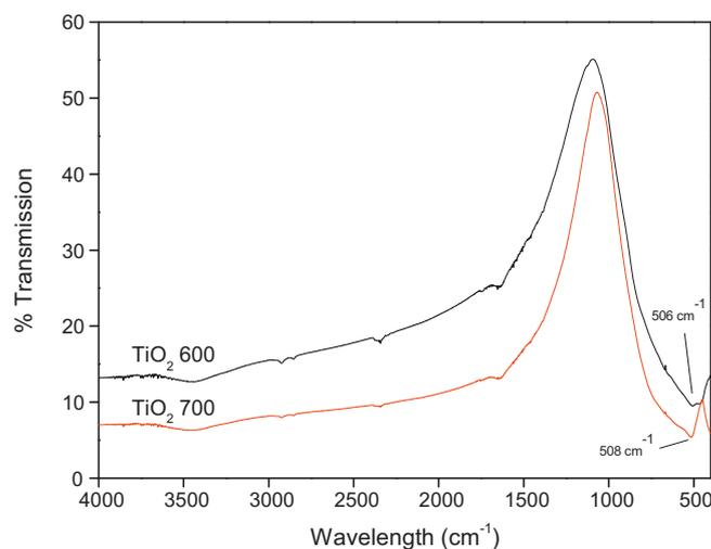
**Fig. 3.** Infrared spectrum of N-doped TiO<sub>2</sub> calcined at 600 °C and 700 °C.
