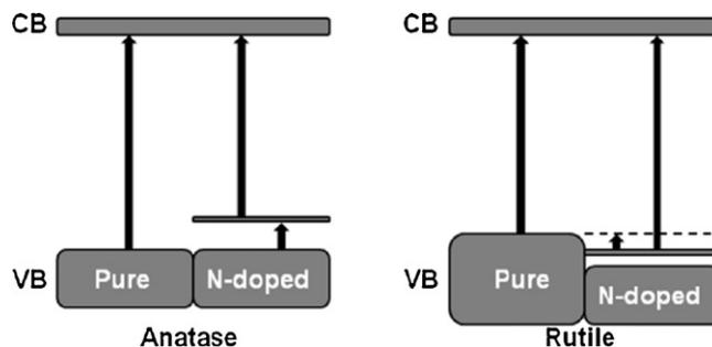
**Fig. 10.** Schematic electronic structure [23] for pure and N-doped anatase and rutile polymorphs of TiO<sub>2</sub>.
