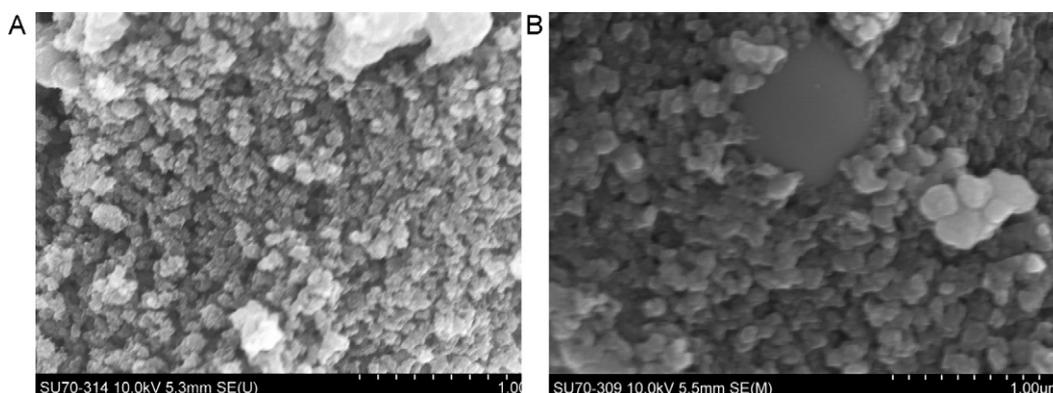
Fig. 8. Scanning electron microscope image of (A) N-doped TiO<sub>2</sub> calcined at 500 °C and (B) undoped TiO<sub>2</sub> calcined at 500 °C.
