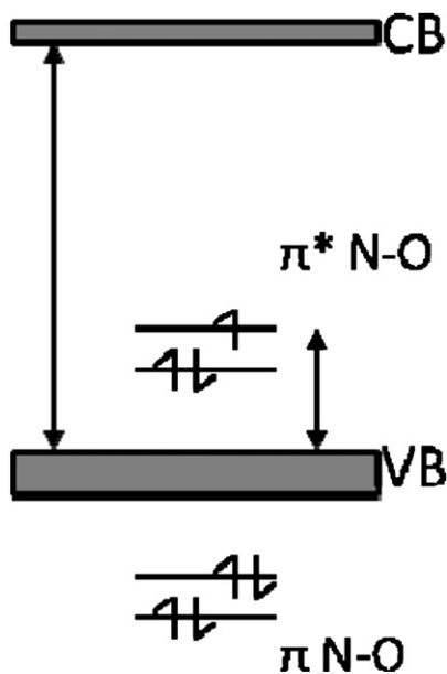
Fig. 7. Electronic structure for interstitial nitrogen doped TiO<sub>2</sub> [25].
