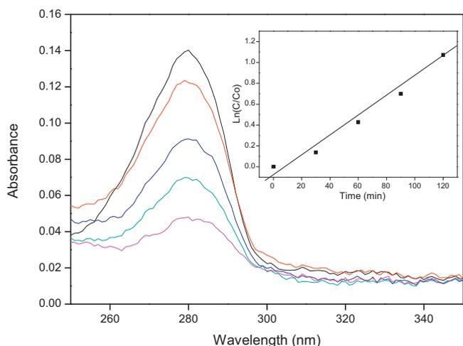
**Fig. 9.** Degradation of 4-chlorophenol using N-TiO<sub>2</sub> calcined at 500 °C under irradiation from solar light in a Q-sun solar chamber.
