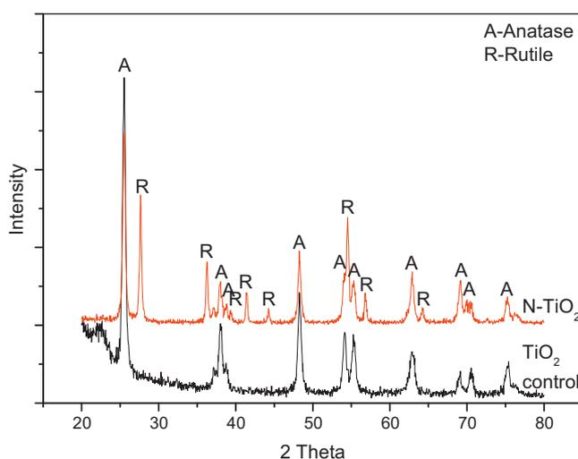
Fig. 1. XRD of TiO<sub>2</sub> control and N–TiO<sub>2</sub> calcined at 600 °C.
