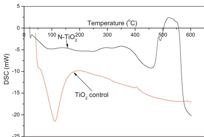
Fig. 4. DSC of doped and undoped TiO<sub>2</sub>.
