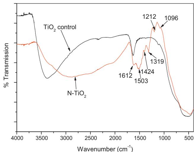
**Fig. 2.** Infrared spectrum of doped and undoped TiO<sub>2</sub> before calcination.
