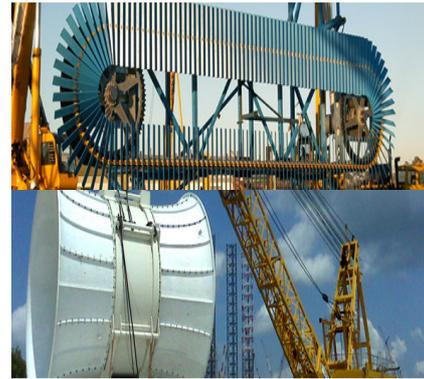
**Figure 10. Nereus Turbine is shown on top, and below is the Solon Turbine[45]**
