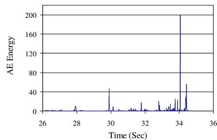
Figure 2: AE energy vs. time at fracture
