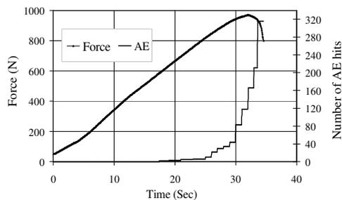
Figure 1: Force & number of AE hits vs. time
