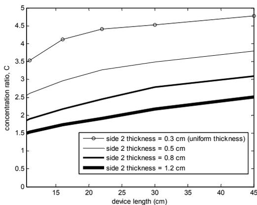
Fig. 9. Concentration ratio ( $C$ ) for device 0.3 cm thick (PV side) x 8 cm wide (see fig. 7). The thickness of side 2 and length of side 1 are varied. The highest  $C$  is obtained for devices of uniform thickness.
