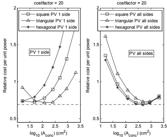
Fig. 5. Relative cost per unit power for different geometries. (a)-PV at one side only. (b)-PV at all sides. The price of concentrator plate per  $\text{m}^2$  was assumed to be 20 times less than that of PV per  $\text{m}^2$  (i.e. costfactor = 20).
