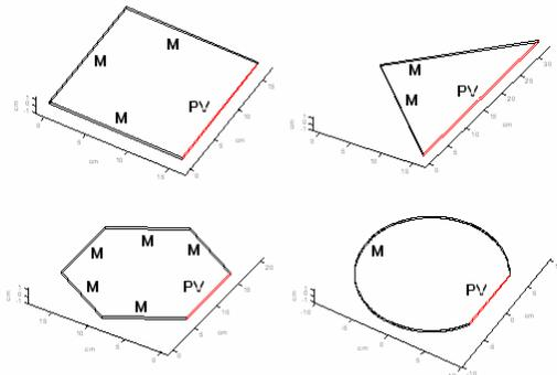
Fig. 3. Square, right angled triangular, hexagonal and circular (PV length=circle radius) devices,  $A_{conc} = 256\text{cm}^2$ . External mirrors (M) may be placed at the non PV sides, as shown here, or PV may be placed at all sides of the device.
