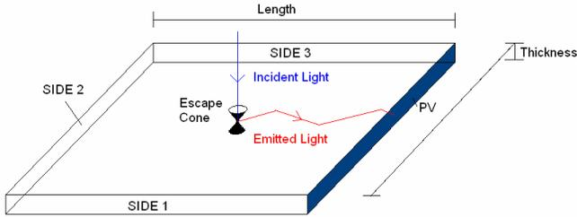
Fig. 1. QDSC consisting of a clear polymer plate doped with QDs, with PV cells attached to one side.
