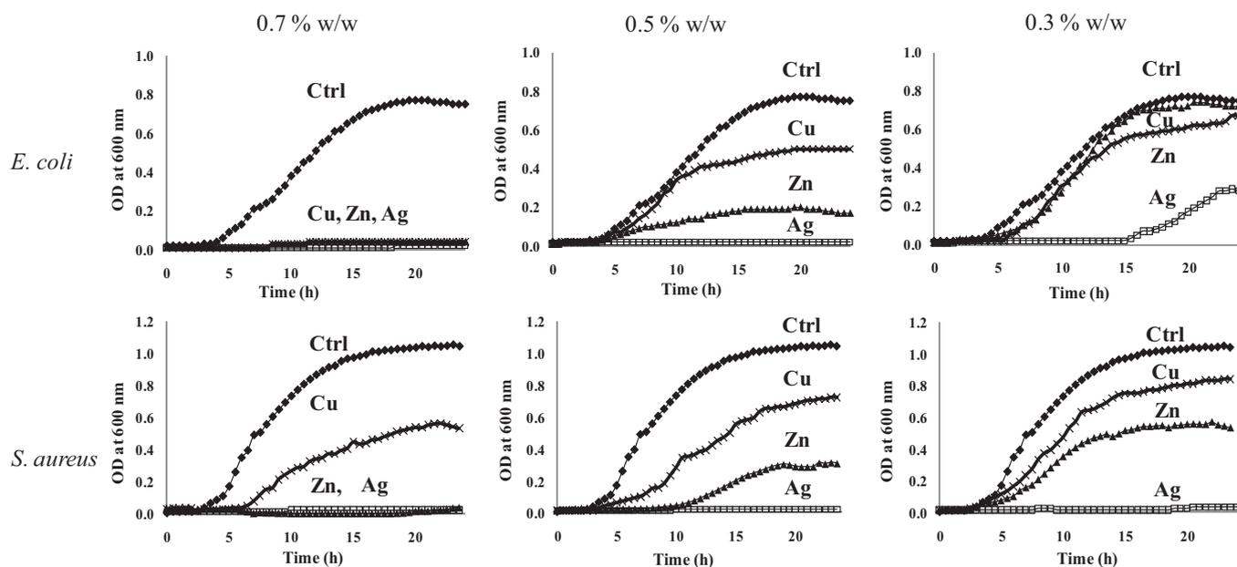
**Fig. 4.** Comparative growth curves of Gram negative *E. coli* ATCC 25922 and Gram positive *S. aureus* ATCC 25923 on the coated sol-gel microtitre well surface containing metal ions (Ag (—■—), Zn (—▲—), Cu (—◆—)) of different concentrations (a) 0.7% (w/v), (b) 0.5% (w/v) and (c) 0.3% (w/v) with respect to control (—●—) (MTEOS coated surface without metal ions) after 24 h of incubation.
