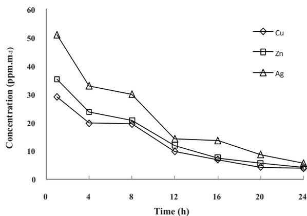
**Fig. 3.** Non-cumulative release rates of Ag, Zn and Cu into fresh DiH<sub>2</sub>O from Ag:MTEOS, Zn:MTEOS, Cu:MTEOS coatings (determined by ICP emission spectrometer).
