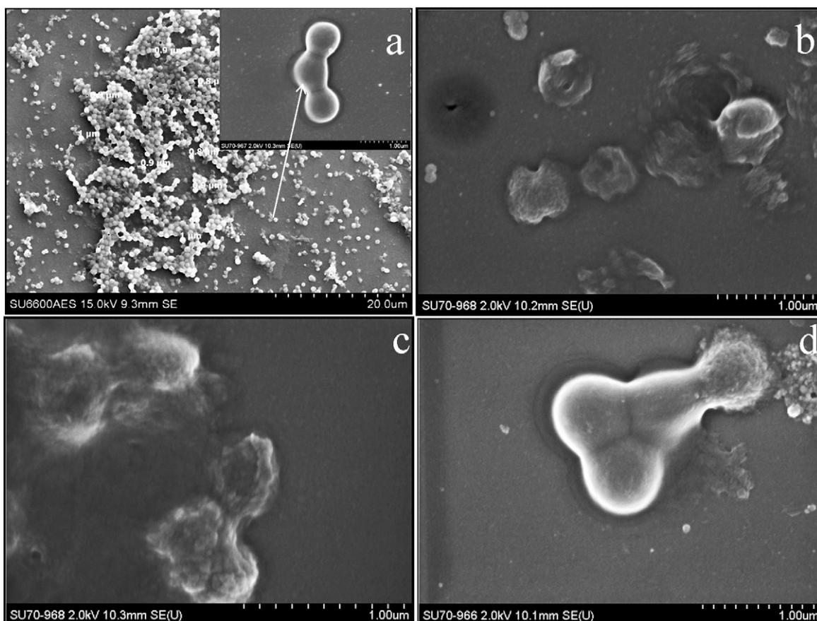
**Fig. 5.** SEM images of *S. epidermidis* CSF41498 on (a) MTEOS coated glass slide without metals, (b) Ag–MTEOS coated glass slide, (c) Zn–MTEOS coated glass slides and (d) Cu–MTEOS coated glass slides, with all MIBC level of metals.
